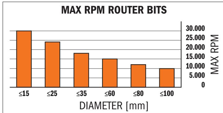
For specific RPM, follow marking on the tool/packaging.
