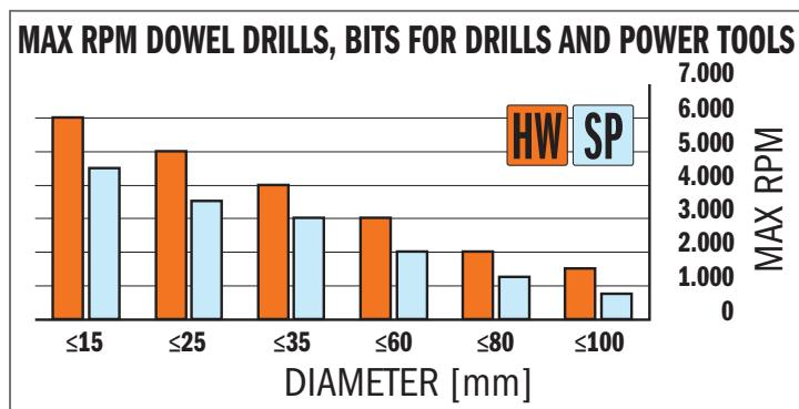
For specific RPM, follow marking on the tool/packaging.
